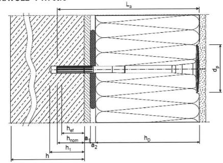
h<sub>nom</sub> = overall plastic anchor embedment depth in the base material
